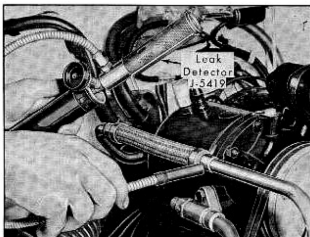
Fig. 16A-15 Testing for Leaks
