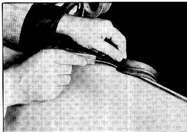
Fig. 3-53 Installing Deck Lid Weatherstrip
