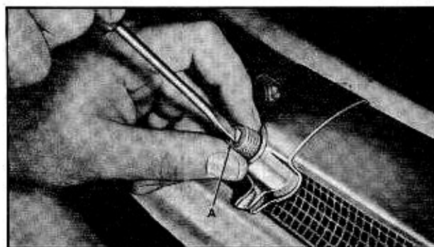
Fig. 3-4 Windshield Wiper Cable Tension Adjustment
