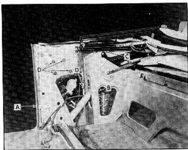
Fig. 3-47 Rear Quarter Window Guide Removal (6267)
